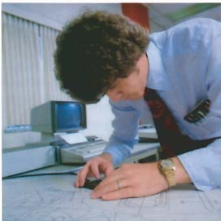
Drafting technician Jack Stone digitizes data points into the System 45 from scale drawings.
