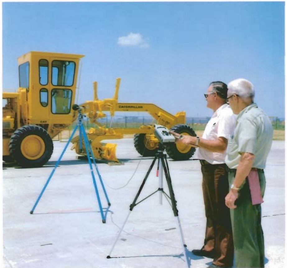
Inspection analyst Donald E. Runyon (left), and quality control analyst Minor Oakley conduct noise level tests on a Motor Grader. Test comparisons between machines help identify defects.
